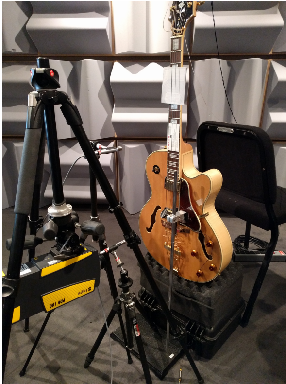
Figure 1: Experimental setup for admittance measurements.
