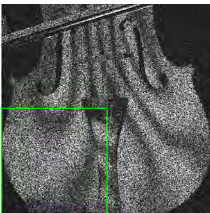
Figure 2: Qualitative ESPI image of the violin. Subtraction intensity of the interference patterns corresponding to a time difference of 4.8 ms (100 frames). The green box features the region of interest.
